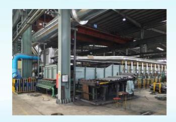
Rotary Heating Furnace (18m)
