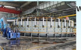
Walking Beam Heating Furnace(24m)
