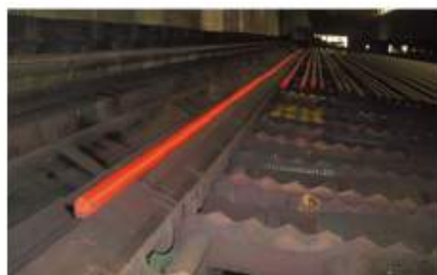
冷床 Cooling Bed
