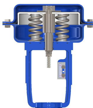
Figure 3. Cross Sectional Drawing AO-3600 Diaphragm Actuator (Reverse Acting)
