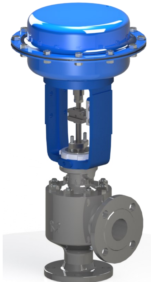
Figure 1. Series 20 angle type globe valve mounted with AO-3600 Pneumatic diaphragm actuator
