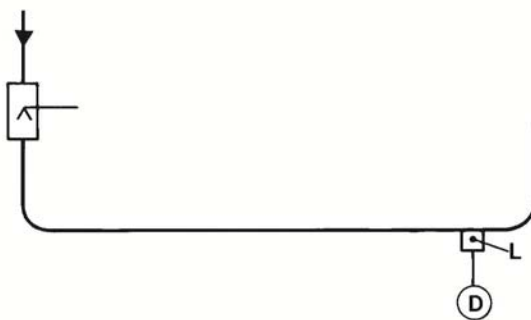
Fig 6 Desuperheater installed in a vertical flow-down pipe
