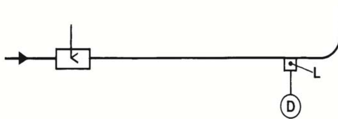
Fig 5 Desuperheater installed in a horizontal pipe
